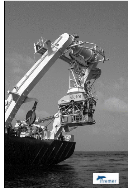
The Remotely Operated Vehicle VICTOR 6000 being lowered from L’Atalante into the Caribbean Sea
